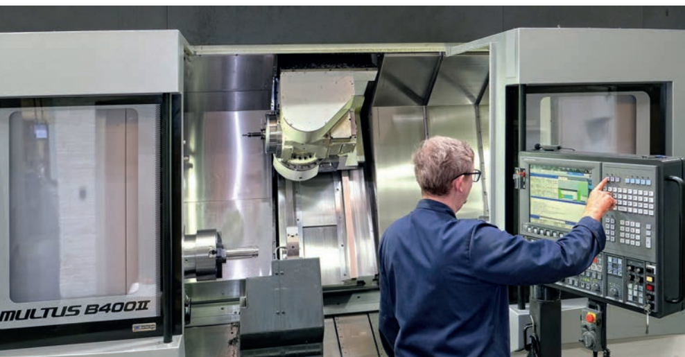
The Okuma Multus B400II-W turn-mill centre with B-axis spindle on the shop floor at EV Engineering. Some parts produced can cost well in excess of £10,000, so this machine will not be automated
