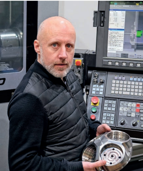
David White in front of the Okuma Multus U3000-2SW turn-mill centre at EV Engineering, High Wycombe. He is holding a machined titanium gyro component for an underwater ROV (remotely operated vehicle)
